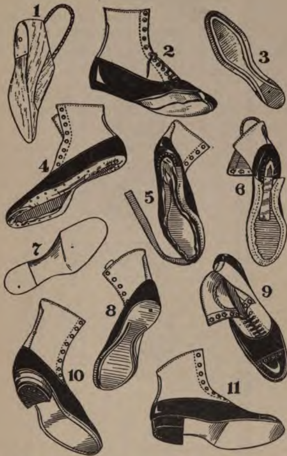
A Goodyear Welt Shoe in the Different Stages of Manufacture
